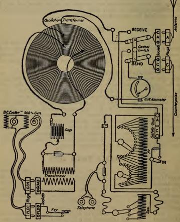
WIRING DIAGRAM, FIELD RADIO PACK SET, MODEL 1913
