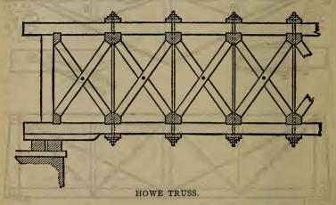
be nailed on or dowels inserted in the ends of the braces for the same purpose. The timbers of the Howe truss are all squaresawed and have no mortises or tenons.
