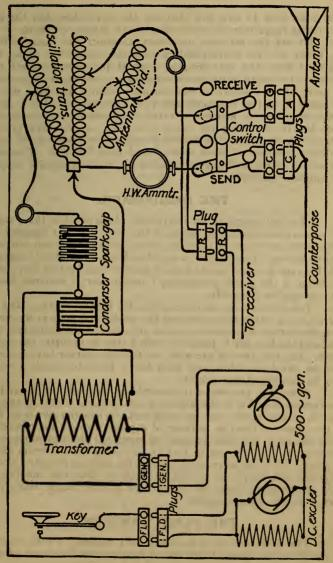
WIRING DIAGRAM, RADIO PACK SET, MODEL 1915
