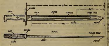
has the following parts: Edge, false edge, back, grooves, point, and tang. The length of the blade from guard to point is 16 inches, the edge 14.5 inches, and the false edge 5.6 inches. The length of the service rifle, bayonet fixed, is 59.4 inches. The weight of the bayonet is 1 pound; weight of rifle without bayonet is 8.69 pounds. The center of gravity of the rifle, with bayonet fixed, is just in front of the rear sight.
